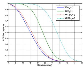
Figure 3: CCDF of capacity versus target rate for selected SNR of channel
