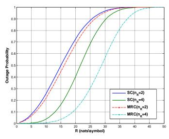
Figure 2: Outage Probability versus target rate for selected SNR of channel
